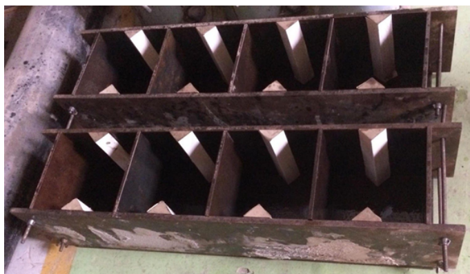
Figure 1 – Steel mold for specimens used in DEWS test.
