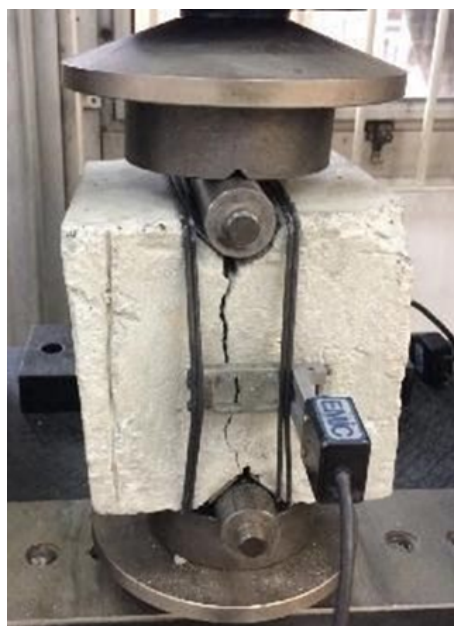
Figure 2 – Setup of the DEWS test.
