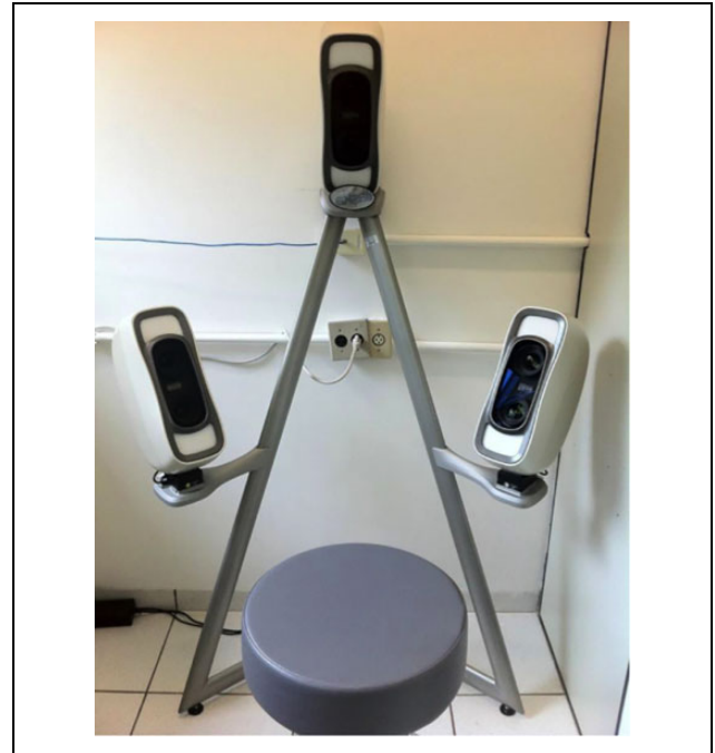
Figure 1. Vectra ® M3 device with capture system with a geometric resolution of 1.2 mm (triangle edge length), a capture time of 3.5 millisecond, on-board modular intelligent flash units, stereophotogrammetry technology, floor stand, stool.
