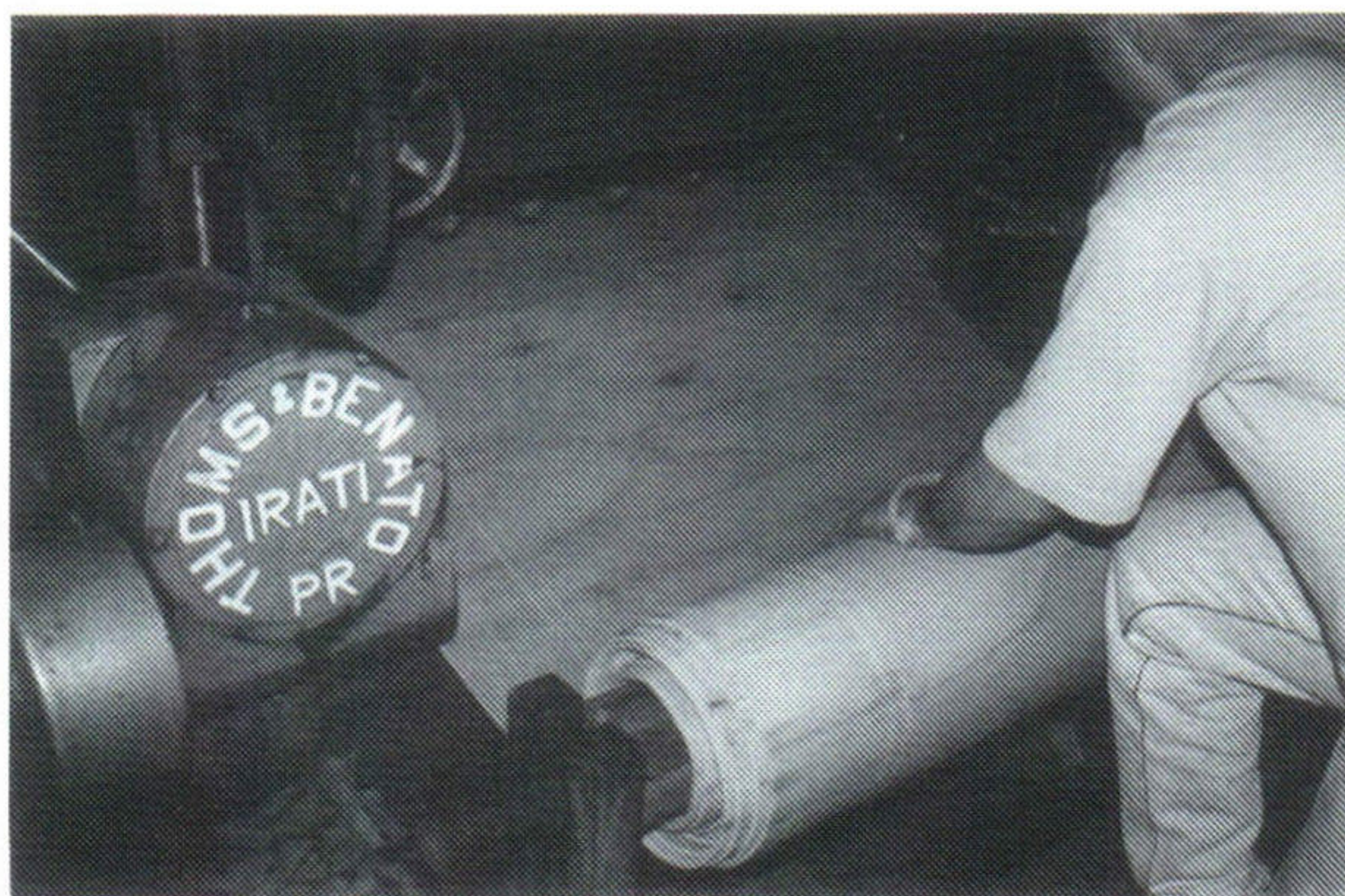
Figure 2. — Lamination process of the logs on a laminating lathe.
