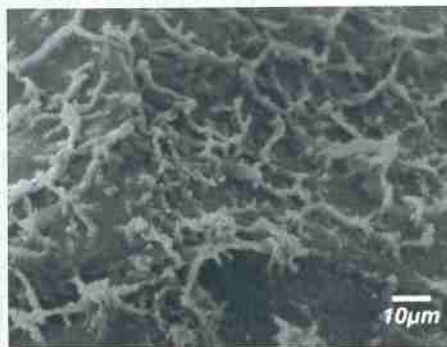
4- Plasma of variable composition (Si, Mg, Fe, Al) covering the apatite grain surface
