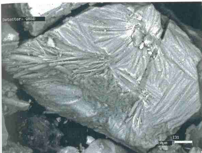
1- Apatite grain showing dissolution cracks 2- Detail of apatite dissolution
