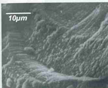
3- Apatite surface covered by secondary aluminum phosphates - crandalite
