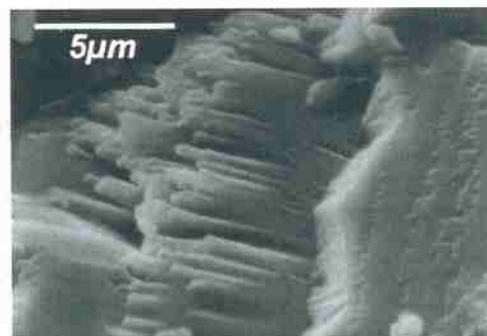
1- Apatite grain showing dissolution cracks 2- Detail of apatite dissolution
