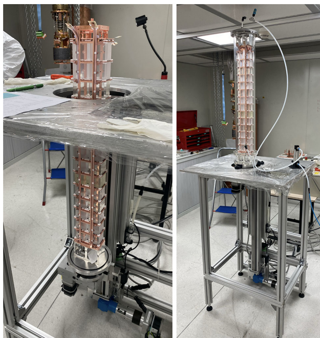
Fig. 4 Tooling for the detector tower assembly. Left: an automated lifting and rotation system allows for a convenient work height during the tower assembly. Right: the circular tower base plate interfaces with an acrylic capsule for transport and storage in an inert atmosphere
