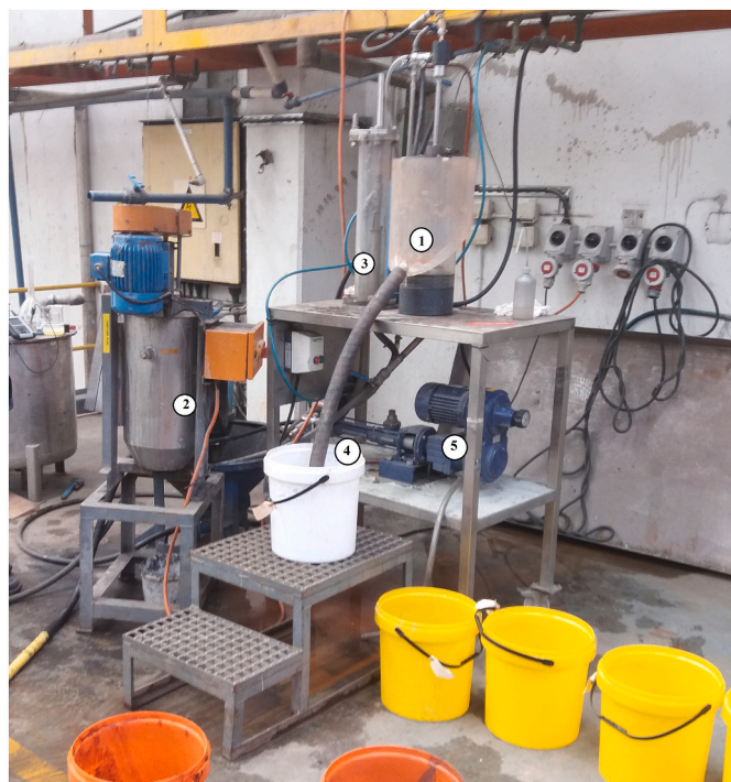
Fig. 1. Pneumatic flotation cell used in the study. (1) Pneumatic reactor; (2) Feed tank; (3) Froth height adjustment; (4) Concentrate collector; (5) Pump.
