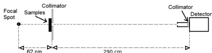
Fig. 1. Experimental setup used in the measurements of the transmitted X-ray spectra through the materials.
