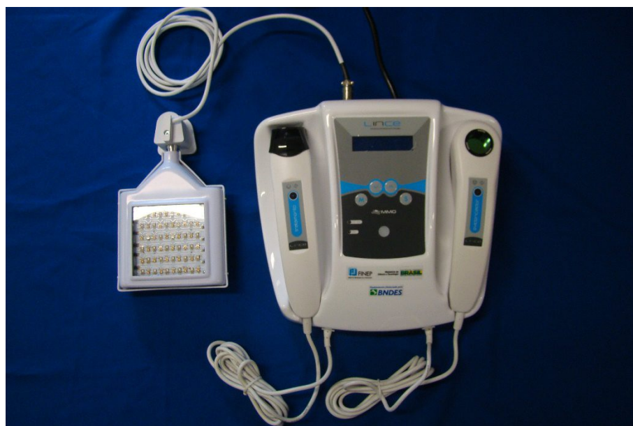
Figure 1 - View of the device platform: a) standard treatment probe; b) large area treatment probe.
