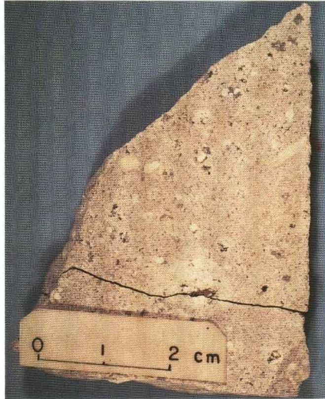
PLATE 3:9-1. Reduced porphyritic phonolite. Note the white alkali-feldspar phenocrysts, microporosities and medium-grey, nearly rectangular pseudomorphs after nepheline. Sample no.: F1/69-1A.
