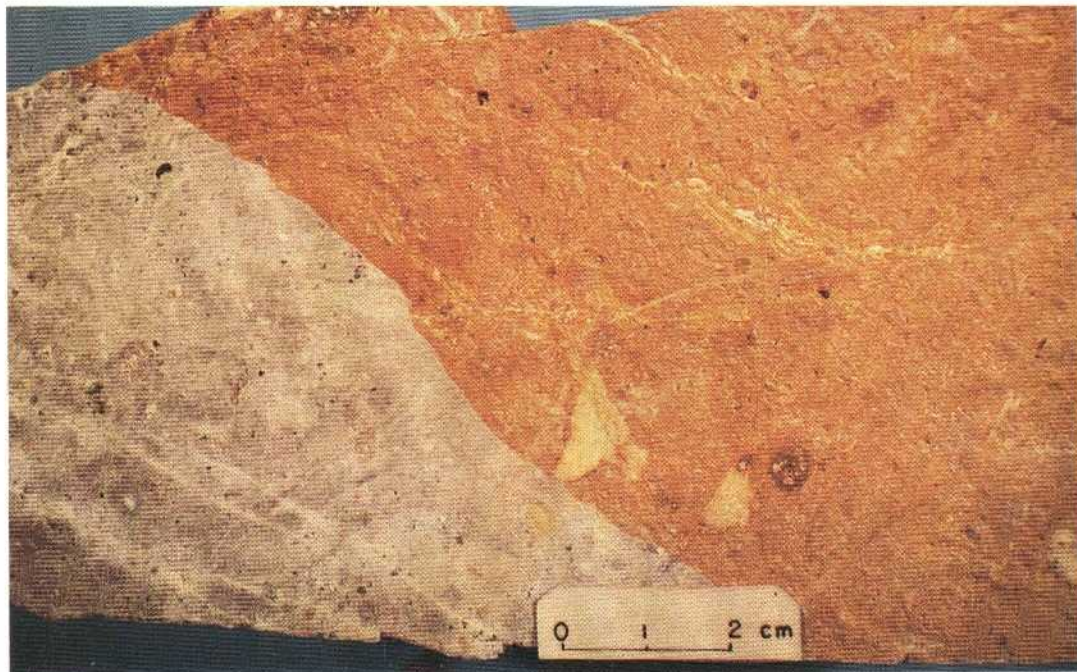
PLATE 3:9-6. Sawn surface of sample illustrated in Plate 3:9-5. Note the sharp redox front in the microxenolithic, fine-grained phonolite. The left-hand part consists of reduced rock, light-grey coloured, and shows microporosities and one (kidney shaped) millimetre-sized pitchblende nodule (upper left, about 1 cm from redox front). The right-hand part of the specimen is oxidised, showing the typical colouration caused by finely disseminated limonite/ HFO-minerals resulting from pyrite oxidation.
