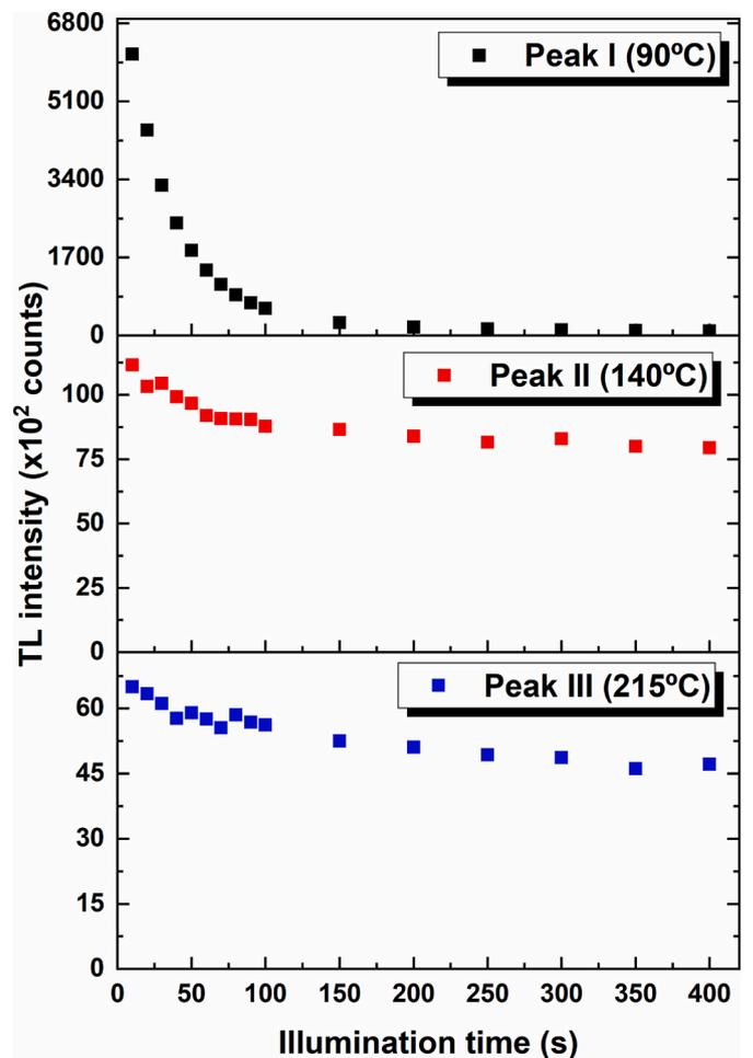
Fig. 3. Influence of previous illumination using blue LEDs on the TL glow peaks. The dots represent the integration of peak I (black solid squares), peak II (red solid squares) and peak III (blue solid squares). (For interpretation of the references to color in this figure legend, the reader is referred to the Web version of this article.)
