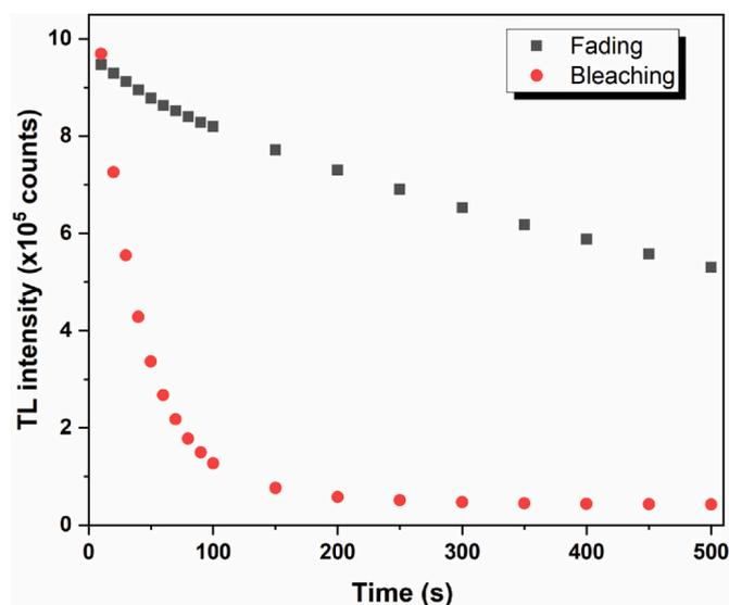
Fig. 4. The integral of the TL curve showing the influence of illumination on the glow peak intensity (red solid circles) in comparison to the effect of pauses in the dark after irradiation on the glow peak intensity (black solid squares). (For interpretation of the references to color in this figure legend, the reader is referred to the Web version of this article.)
