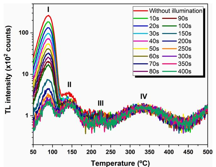
Fig. 2. Influence of previous illumination on the TL glow peaks. A semi-logarithmic scale is used for better visualization.
