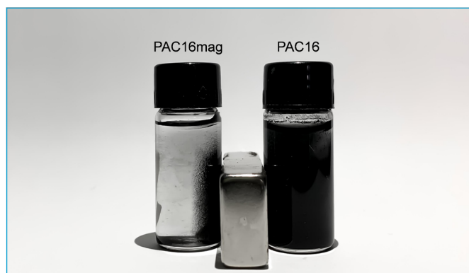
Figure 3 – Magnetic attraction of PAC16mag compared to non-magnetic PAC16.
