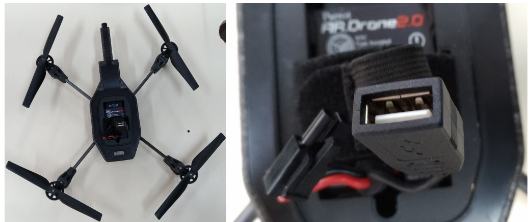
Figure 7. The Parrot AR.Drone 2.0 without its hull, highlighting its USB port.
