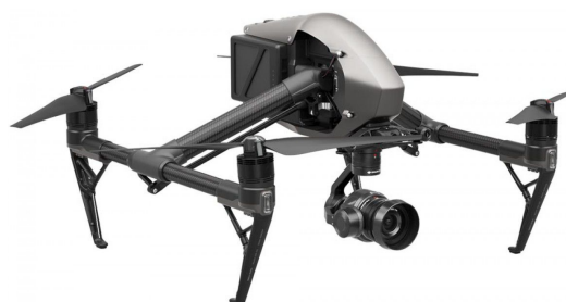
Figure 1. DJI Inspire 2, a mini UAV weighing around 3.3 kg and capable of a flight time up to 27 min [17].
