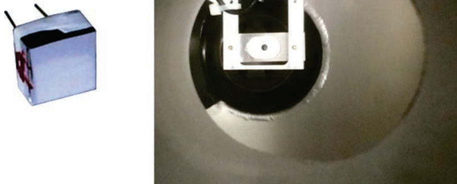
Fig. 56. Left: the CsI(Tl) crystal used for the radiation hardness test. Right: the mechanical support hosting the crystal and an alumina beam monitor to check the beam alignment and focusing.
