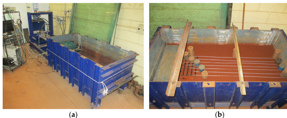
Figure 2. Large-scale pullout test apparatus: (a) overall view; (b) inextensible wires fixed along the GGR.
