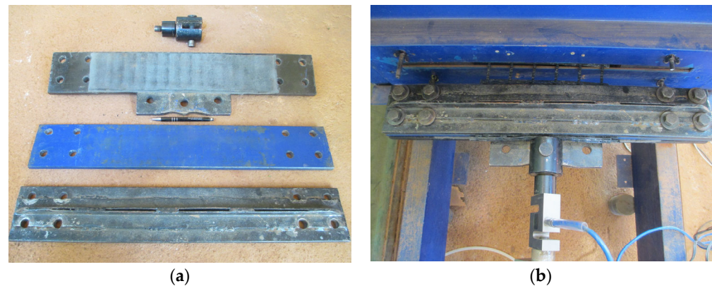
Figure 6. Clamping system: (a) clamp apparatus; (b) installed clamp system.
