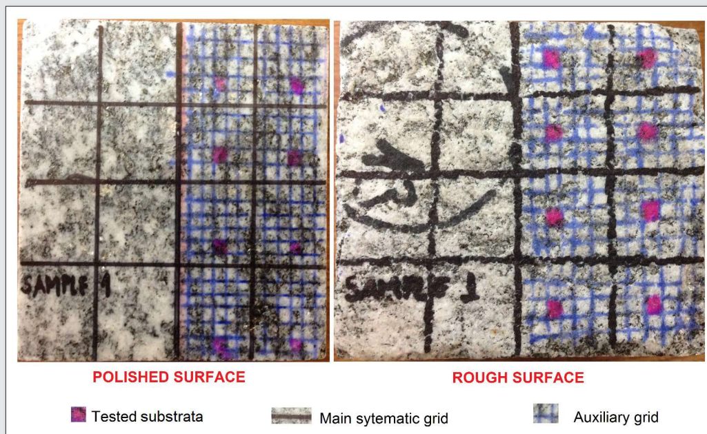
Figure 5. SRS applied to 5 x 5 cm plates of both polished and rough surfaces – Sample 1. Schematic drawing covers only half plates but the measurements were conducted in full, totalling 16 substrata on each surface.
