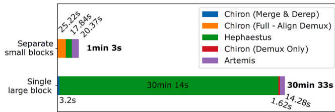
Fig. 8. Decoding time performance improvement when the sequencing dataset is partitioned, possible because of the block structure (simulation scenario). When sequencing data is processed as a single large block (as in literature methods), the clustering time (Hephaestus) is drastically longer (the long green bar is out of scale), and the overall process is approximately 29 times longer than the same method with block partitioning (as proposed).
