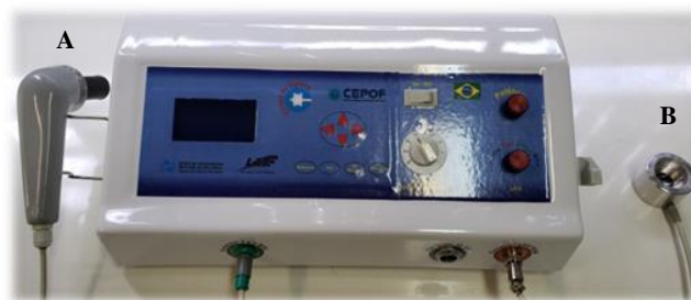
Figure 1. Ultrasound (A) and blue LED light device (B) developed by the Technical Support Laboratory, IFSC, USP.
