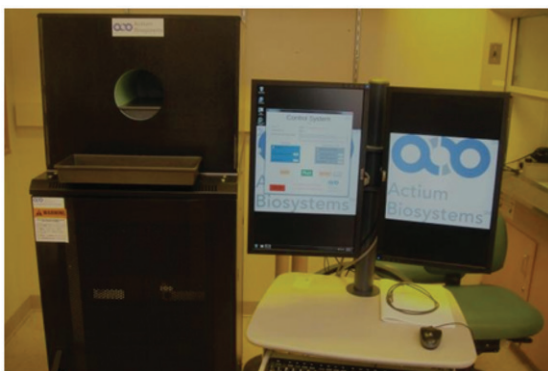
Figure 1. Induction coil chamber and power supply of a small animal magnetic field hyperthermia system (Actium Biosystems) with thermal monitoring and control console.
