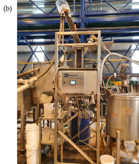
Fig. 6. Schematic representation of the Reflux Classifier (a) and image of the pilot-scale Reflux Classifier (b).
