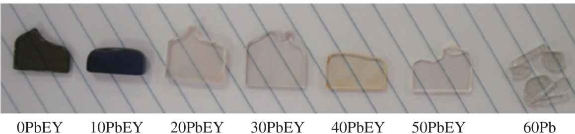
Figure 1. Glass samples obtained in the ternary system \text{NaPO}_3-\text{WO}_3-\text{PbF}_2 .
