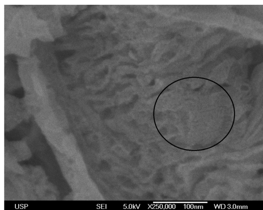
Fig. 11. TEM image of the ZeCe-2 sample with slit like pores and circular pores (circle).
