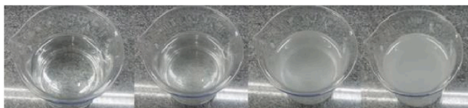
Fig. 2. Gradual calcium carbonate formation in the solution at 25 °C.
