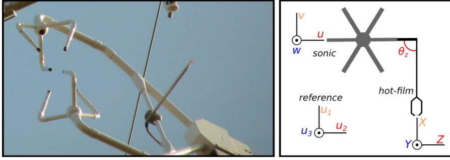
Fig. 1 Left: picture of the sonic and hot-film sensors in the field (hot-film attached to the vertical support of the sonic arms in a 90° angle). Right: top view of the coordinate system of the sonic \langle u, v, w \rangle (pointing westward) and hot-film \langle X, Y, Z \rangle (pointing southward). We define the reference coordinate system as \langle u_1, u_3, u_2 \rangle and redefine the sonic and hot-film data accordingly.
