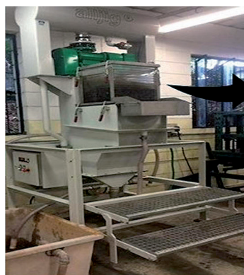
Figure 4 Jig device details used in the test.
