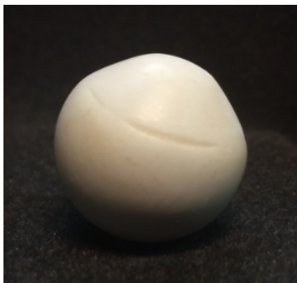
Fig. 8. Machining pattern resulting from the application of inverted angular velocities to lower plates.
