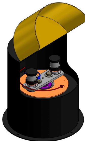
Figure 3. Sketch of the planetary mill designed with a protective external structure.
