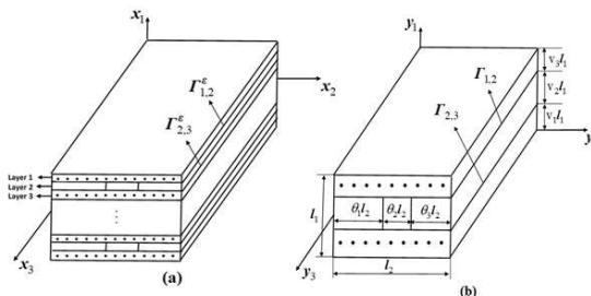
**Figure 1** – Analytical model: (a) laminated composite; (b) unit cell with delamination in the layer 2 [1].
