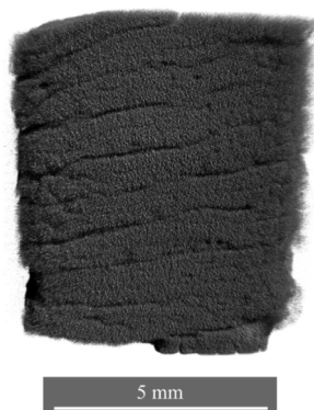
Figure 2. Micro-CT image of the QC sample leached in NaOH alkaline solution for 48 h. The scale bar represents 5 mm.
