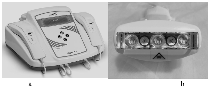
Figure 1 – A piece pf equipment for photobiomodulation with lasers and LEDs, with acrylic tip (diode cluster) Venus (MMOptics, São Carlos, Brazil). In "b", a detail of one of the handles where it is possible to observe the presence of 3 LEDs interspersed by 2 laser diodes: in one handle the device has 3 blue LEDs with 2 red LEDs, and in the other one it has 3 LEDs infrared lasers with 2 infrared lasers (personal archive).
