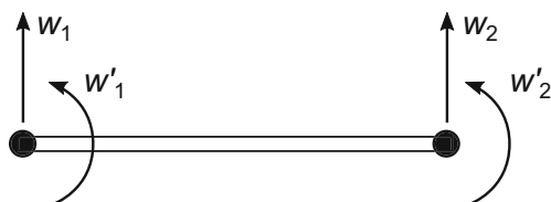
Fig. 2 Two-node/four-dof Bernoulli–Euler beam finite element
