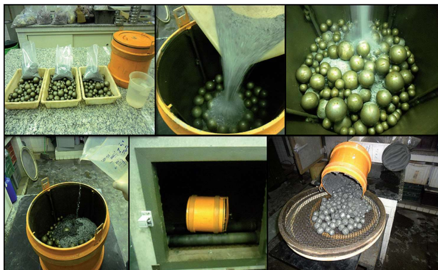
Figure 1 Test grinding ball mill sequential procedure.
