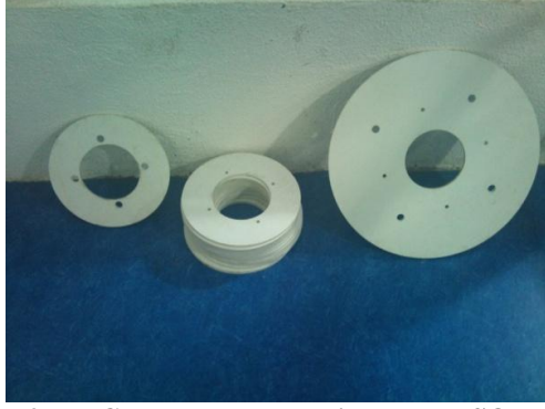
Figure 2- PVC plates used to build the MPSO models.
