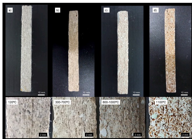
Fig. 8. Stereoscopic images of samples of MPMB thermal insulator thermally treated at different temperatures (a) 120 °C, (b) 300–700 °C, (c) 800–900 °C, and (d) 1000–1100 °C detailing the lamination cracks formed during heating and the surface aspect.
