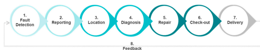
Figure 1. Conceptual framework of the traditional reactive maintenance process.
