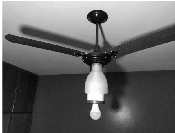
Figure 10. Final lighting sensor.
