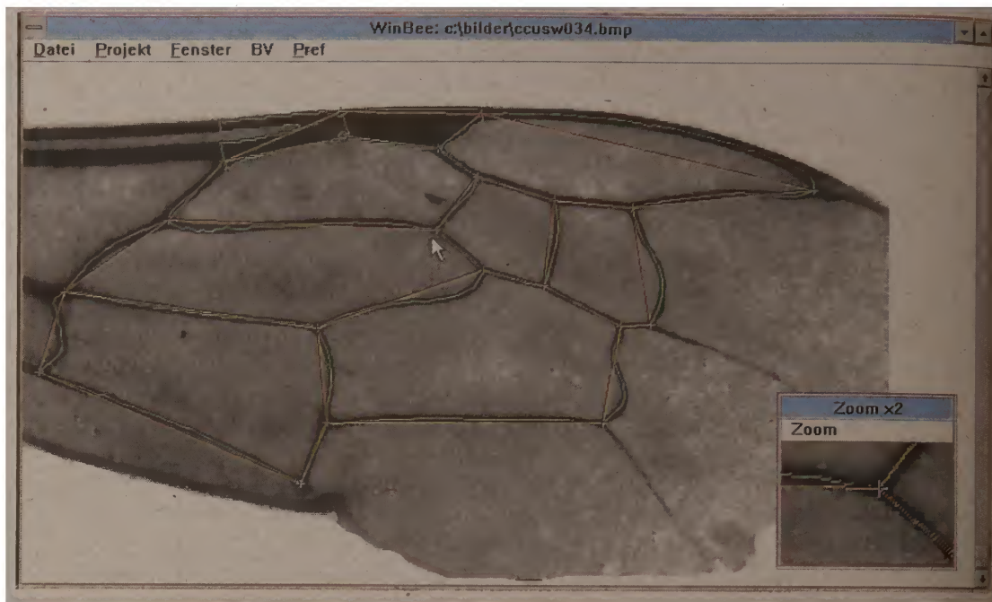
FIGURE 3: From the wing image (curved lines) the venation graph is extracted. This is the graph in which all vein junctions are connected by straight lines
