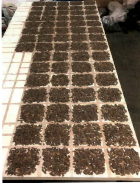
FIG. 2 - Material spread on the table for the heterogeneity test
