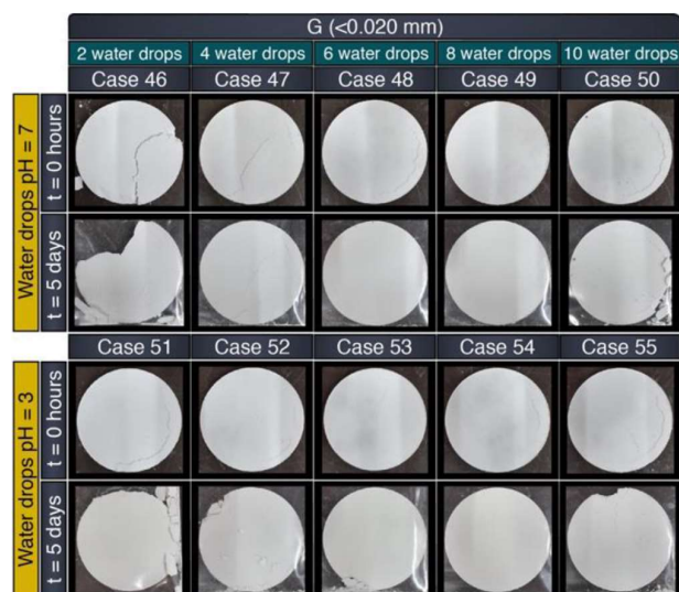
Fig. A.5. Constructed discs aiming to study the influence of pH and quantity of water drops on the carbonate consolidation. Particle size ( <0.020 mm) and drying temperature 25^{\circ}\text{C} .
