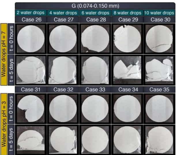
Fig. A.3. Constructed discs aiming to study the influence of pH and quantity of water drops on the carbonate consolidation. Particle size (0.074–0.150 mm) and drying temperature 25 °C.
