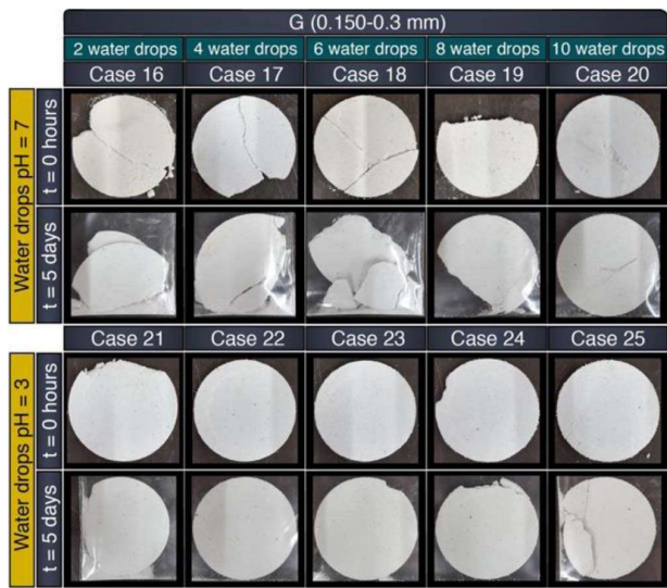
Fig. A.2. Constructed discs aiming to study the influence of pH and quantity of water drops on the carbonate consolidation. Particle size (0.150–0.3 mm) and drying temperature 25 °C.
