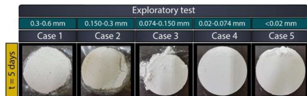
Fig. 6. Exploratory test discs aiming to study the influence of particle size on material consolidation and drying temperature 25 °C.
