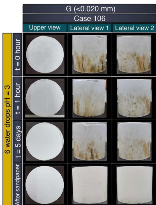
Fig. 10. Synthetic carbonate plug of real size, using particle size (<0.020 mm), six water drops with pH 3, uniaxial compression and drying temperature 100 °C for 1 h.
