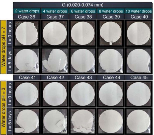
Fig. A.4. Constructed discs aiming to study the influence of pH and quantity of water drops on the carbonate consolidation. Particle size (0.020–0.074 mm) and drying temperature 25 °C.
