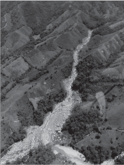
Figure 9. Aerial view photograph of December, 2014: View from downstream of the T2 section, highlighting the erosion and deposition areas along the channel under confined flow conditions.
