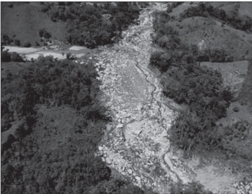
Figure 10. Aerial View of the transition area T2 / T3, from upstream: notice number and size of materials deposited in the stretch. The drainage in this part had a width of about 2 m before the passage of the flow.
