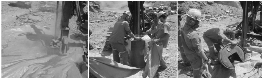
Figure 2 The two sampling procedures for particle size and grade distribution analysis
