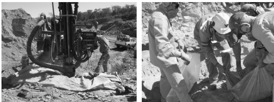
Figure 1 The selected blast hole sampling procedure for MTM reconciliation
