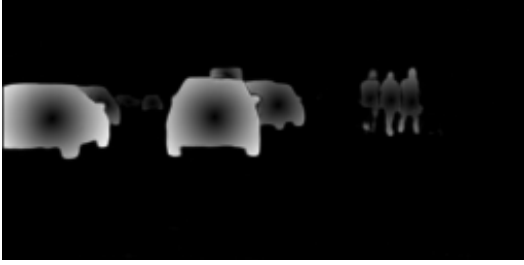
Fig. 2: DCME magnitude map. Large objects present longer vectors close to their borders. Car contours are brighter than people contours.
