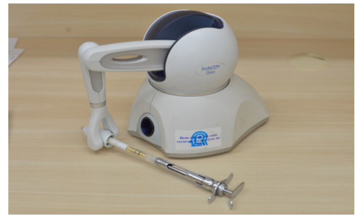
FIGURE 10. Haptic device with Carpule syringe - instrument used by dentists in the anesthesia procedure [36].
