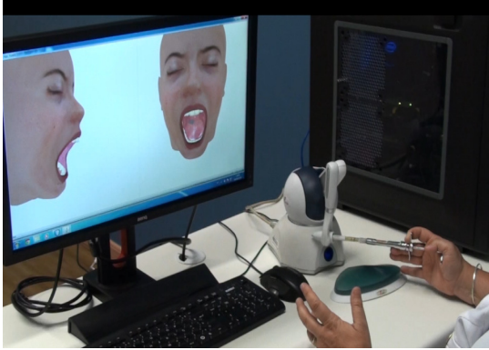
FIGURE 1. User interaction with a haptic device in a VR-based system for dental training using two viewpoints of the same virtual scene [3].
