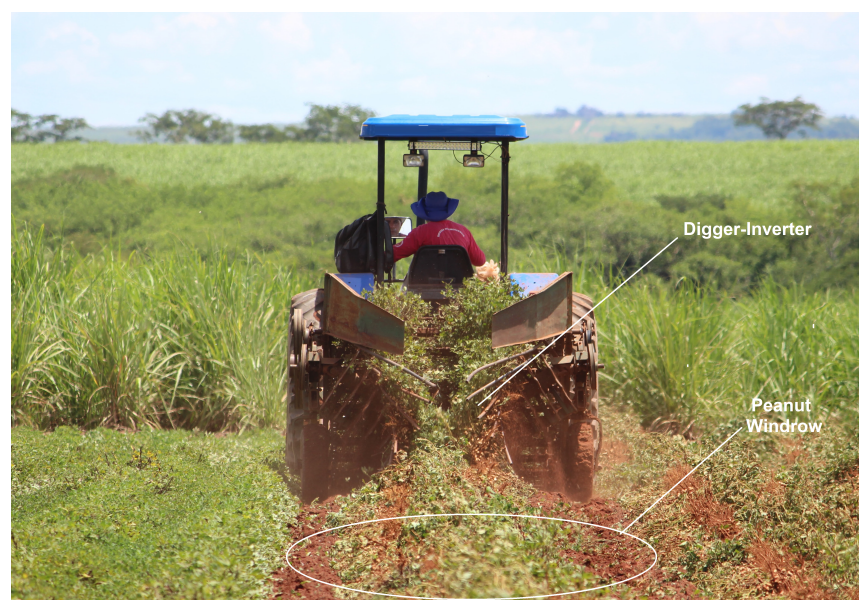
Figure 2. Operation of the digger–inverter, forming the windrow [33].
