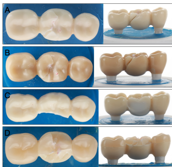
Figure 5. Representative samples of all Groups after single-load-to-fracture assessment. Light microscopy shows (A) occlusal and side view of Group Z-HT, bulk fracture of FDP within the distal connector (B) Group Z-ST, bulk fracture of FDP within the distal connector (C) Group FL, bulk fracture without involvement of the distal connector (D) Group RL, chipping fracture of PICN and bulk fracture of the zirconia framework.
