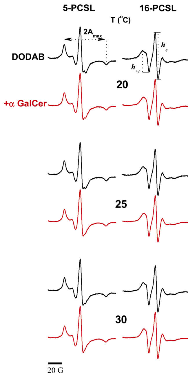
Fig. 3. Effect of 0.2 mM \alpha -GalCer on ESR spectra of 5-PCSL and 16-PCSL embedded in 2 mM DODAB bilayers at temperatures below the gel-fluid transition. The maximum hyperfine splitting ( A_{\text{max}} ) and the amplitudes of low ( h_{+1} ) and central ( h_0 ) fields are indicated. Total spectra width is 100 G.
