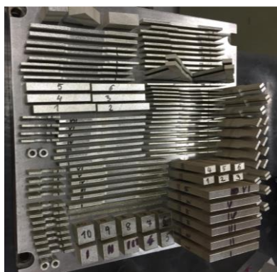
Figure 1. Selective laser melted specimens on substrate plate to be removed after build.
