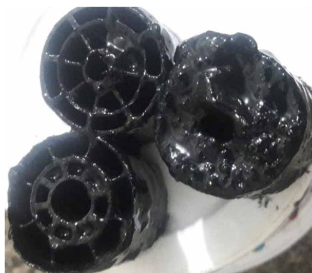
Figure 2 | Low-density polyethylene ring used as support material after operational time.
