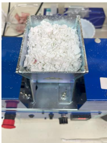
Figure 1: Sample of material crushed in the extruder
