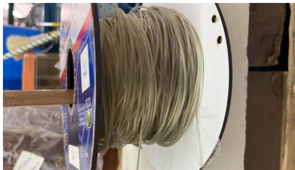
Figure 2: Sample of the EPS filament produced.
