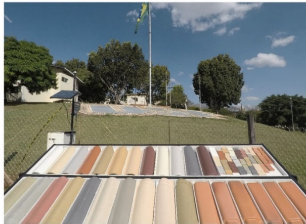
Figure 3. Weathering rack finished and in operation.
