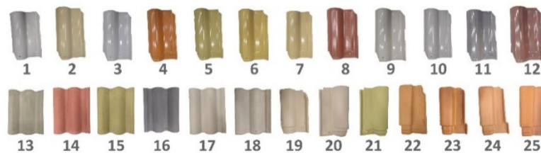
Figure 1. Selected tiles. 1 to 12 - glazed ceramics; 13 to 18 – concrete; and 19 to 25 - pigmented or conventional ceramic.
