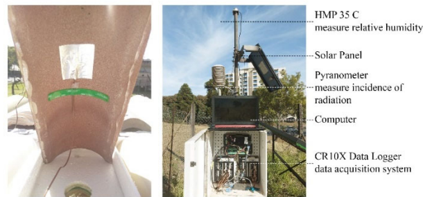
Figure 4. a) Thermocouple position b) Supplementary measuring system and rack feed.
