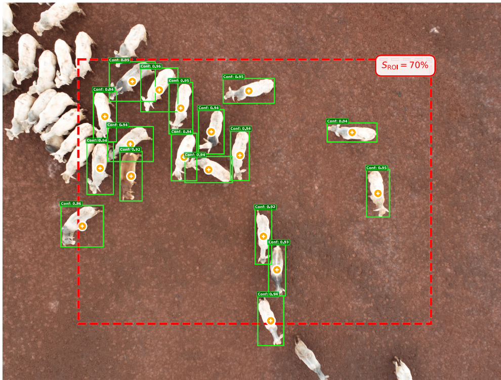
Fig. 3. Example image illustrating ROI and cattle centroid filtering. The red dashed box denotes the ROI boundary ( S_{ROI} = 70\% ). Green boxes indicate detected standing cattle whose centroids lie within the ROI. Orange circles with white crosses mark bounding-box centroids. Cattle without green bounding boxes were detected by YOLOv11s but excluded by the ROI and centroid filtering criteria.
