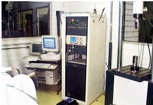
Figure 1 – Standard reaction rig for mechanical tests: maximum load capacity of 105kN.
